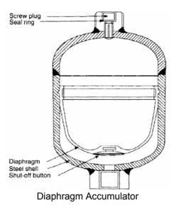
Diaphragm accumulators come in limited volumes, have most of the advantages of bladder-type units but can handle compression ratios of up to 8:1. But their performance can sometimes be affected by gas permeation across the diaphragm.
