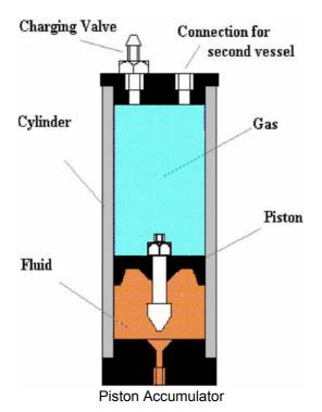
But piston accumulators also require a higher level of fluid cleanliness than bladder units, have slower response times (greater than 25 milliseconds), especially at lower pressures and exhibit hysteresis. This is explained by the static friction of seal which has to be overcome, and the necessary
